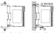
Pull the rail lock at the top and bottom of the module.
