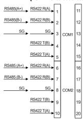
•TMHC-22EE [Ethernet communication module]
