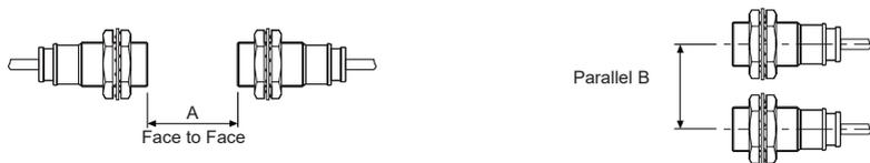
When sensors are mounted on metallic panel, it must be prevented sensors from being affected by any metallic object except target. Therefore, be sure to provide a minimum distance as below chart indicates.
