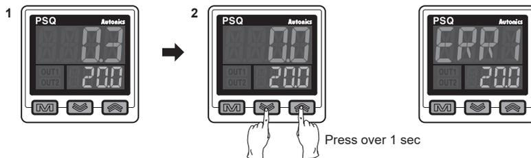
※If executing zero-point adjustment when external pressure over  $\pm 5\%$  of rated pressure is applied, **ERR 1** flashes five times during pressing the keys. Remove external pressure and execute zero point again.
