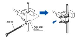
• When additional zip ties are necessary, please use zip ties with a thickness 2.5 mm or smaller as shown by (A) in the diagram below.
