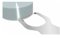
Wafer mapping with the NF-RG01 retro-reflective type.
