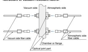
Leakage amount: 1.33 × 10<sup>-10</sup> Pa·m³/s [He] or less
