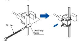
$\cdot$  When additional zip ties are necessary, please use zip ties with a thickness 2.5 mm or smaller as shown by a in the diagram below.
