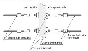
Leakage amount: 1.33 × 10<sup>-10</sup> Pa·m³/s [He] or less
