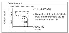
※Each bit of output has the same circuit.
