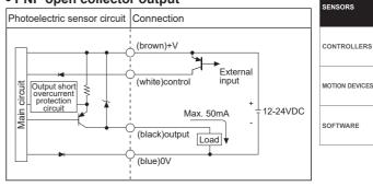
// If short-circuit the control output terminal or supply current over the rated specification, normal control signal is not output due to the output
