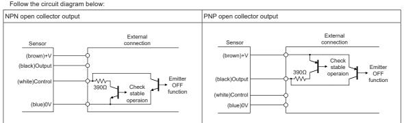
\*When using the emitter OFF function and check stable operation function simultaneously, the transistor used should be able to open and close 50mA/10V and resistance should be over 1/8W. Failure may cause product damage.
