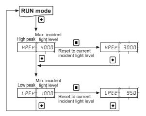
① Press the • (MODE) key for a sec to monitor max/min incident light level.
