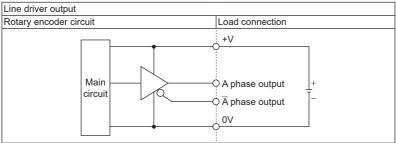
XAll output circuits of A,  $\overline{A}$ , B,  $\overline{B}$ , Z,  $\overline{Z}$  phase are the same.
