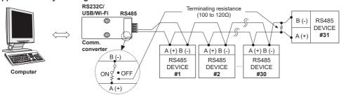
%It is recommended to use Autonics communication converter; SCM-WF48 (Wi-Fi to RS485·USB wireless communication converter, sold separately), SCM-US48I (USB to RS485 converter, sold separately), SCM-38I (RS232C to RS485 converter, sold separately). Please use twisted pair wire, which is suitable for RS485 communication, for SCM-WF48 and SCM-US48I.
