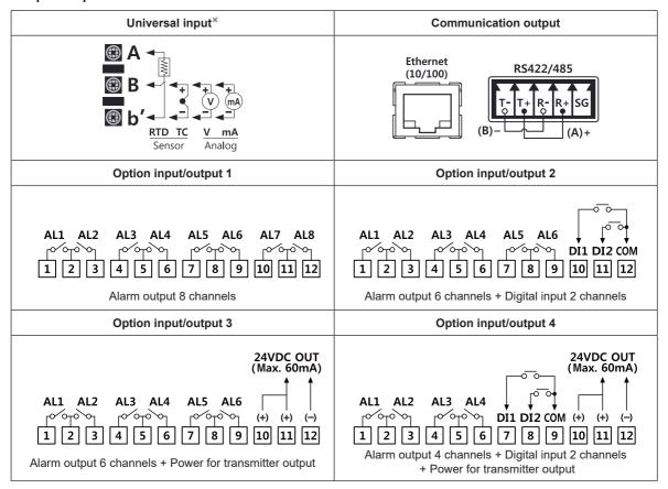
$\times$  In case of current input, connect 250 $\Omega$  resistance at external part.
