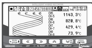
Press the **MENU ENTER** key once in RUN mode and it enters to QUICK MENU. QUICK MENU consists of usually used parameters for quickly parameter setting.
