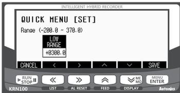
Press the NEXT (**MENU ENTER**) key once and it moves to QUICK MENU [2]. Press the SET (**<<**) key using (**<<**) (**AL RESET**) (**FEED**) (**DISPLAY**) (**ME MO**) keys to set low-limit input range[LOW RANGE] as 300. Press the **MENU ENTER** key.
