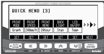
Press the NEXT (**MENU ENTER**) key once and it moves to QUICK MENU [3]. Press the SET (**<<**) key and set standard record speed [PRINT SPEED] as 240mm/h. Press the **MENU ENTER** key.
