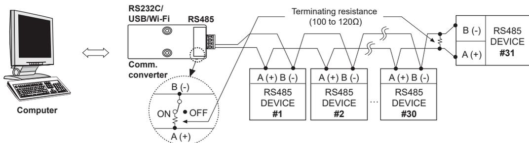
※ It is recommended to use Autonics communication converter; SCM-WF48 (Wi-Fi to RS485-USB wireless communication converter, sold separately), SCM-US48I (USB to RS485 converter, sold separately), SCM-38I (RS232C to RS485 converter, sold separately). Please use twisted pair wire, which is suitable for RS485 communication, for SCM-WF48 and SCM-US48I.
