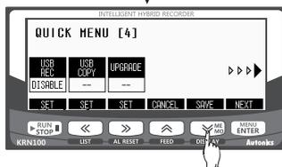
After completing the setting, press the **SAVE (MR MD) (DISPLAY)** key at QUICK MENU [4] and save the settings. It returns to RUN mode.
