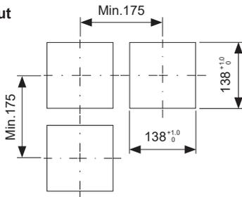
※ Use a steel plate which is 2 to 8mm thickness.
