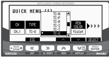
Press the SET (**<<**) key at QUICK MENU[1] and below screen is displayed. Set input type[TYPE] as TC-U by pressing SET (**<<**) (**FEED**) (**ME MO**) (**DISPLAY**) keys and press the **MENU ENTER** key.
