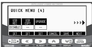
Press the NEXT (**MENU ENTER**) key once and it moves to QUICK MENU [4]. Press the SAVE (**ME MO**) (**DISPLAY**) key to save the settings of QUICK MENU [1] to [4] and it returns to RUN mode.
