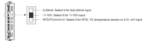
This unit is multi input product. Select the proper input with the input type selection switch and select this input type in l n P in program mode. The setting of input type selection switch and the input type l n P parameter should be same and it can display the proper measurement value. Factory default is 0-20mA.
