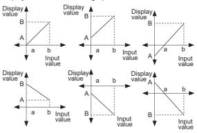
Display scale function is able to change display value for max./min. measured input by setting high limit scale [H-5L] and low limit scale [L-5L] in program mode.
