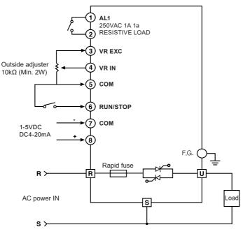
XR, S, U terminals are at the bottom of the unit. For wiring terminals, open the front cover.
