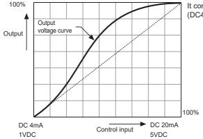
It controls phase angle proportional to control input (DC4-20mA or 1-5VDC) level.
