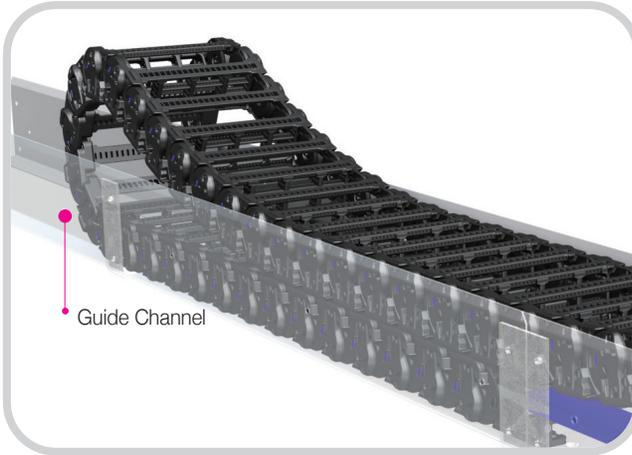
For long stroke applications the guide channel is applied to ensure that the Shift Chain Sliding Chain stays on track and to ensure safety during operation. With the application of a rubber pad on the channel floor, noise is reduced to a minimum. Guide Channels are made of Steel + Zn and can be customized with SUS material .
