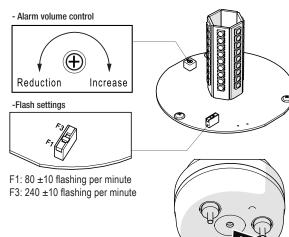
\* When installing a light with built in buzzer, please allow minimum of 5mm space from the surface to the base of unit.
